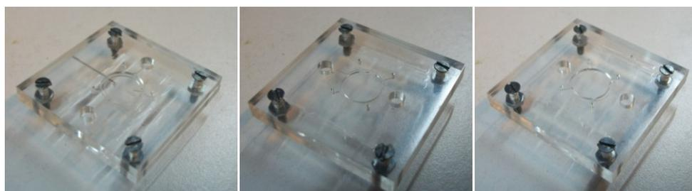
Figura 5.48: Moldes de PMMA
