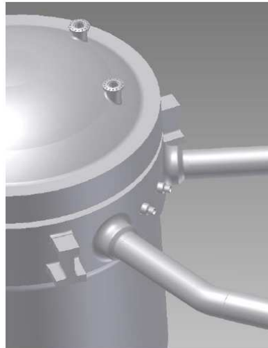
Figure 7.1: Detail of the nozzle weld that connects the reactor pressure vessel and the cold leg.
