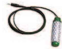
Figura 4.1: Sensor Matricial Granular (Watermark).
